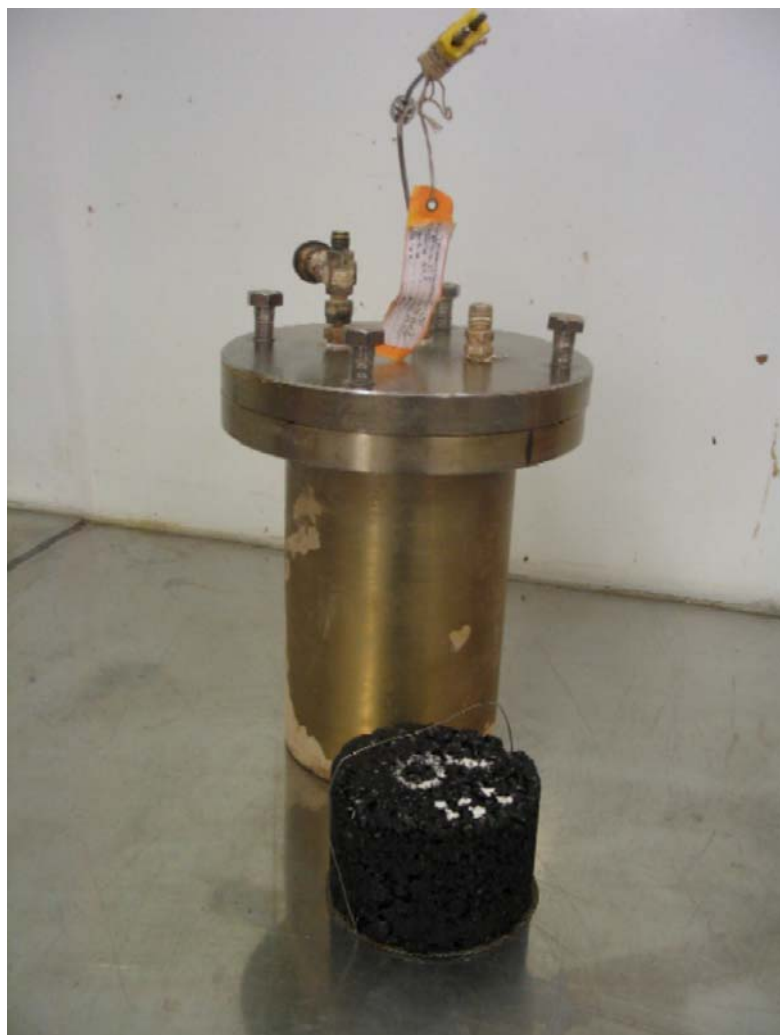
Figure 2.2 Pressure vessel used to oxidise OGPA specimens.
