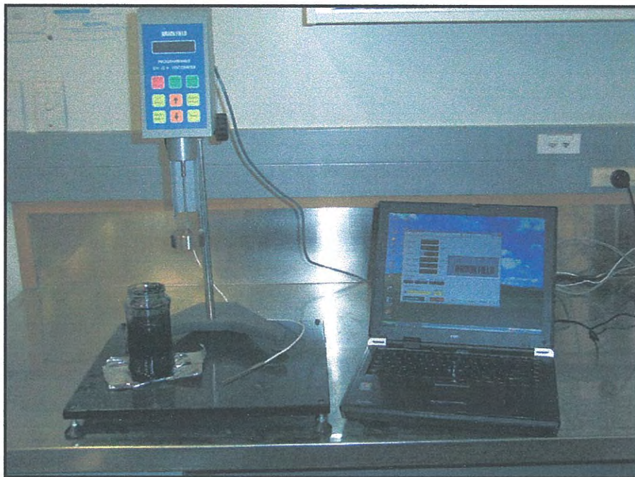
Figure 2.2 Brookfield rotational viscometer used for quantifying foam quality.
