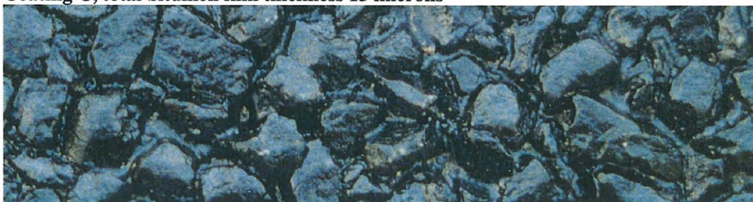
Coating D, total bitumen film thickness 110 microns
