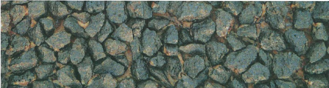
Coating B, total bitumen film thickness 4 microns
