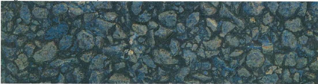
Coating A, total bitumen film thickness 1 micron
