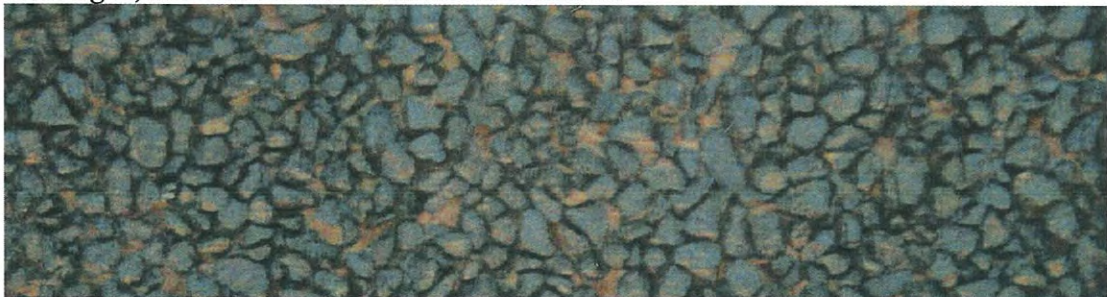
Coating B, total bitumen film thickness 4 microns
