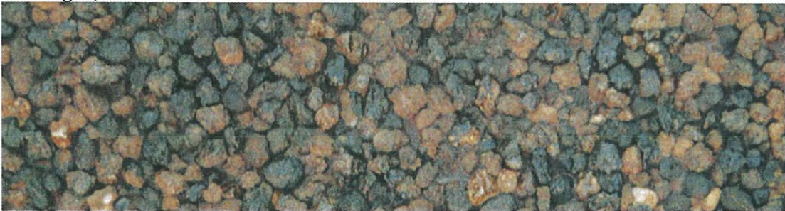
Coating B, total bitumen film thickness 4 microns
