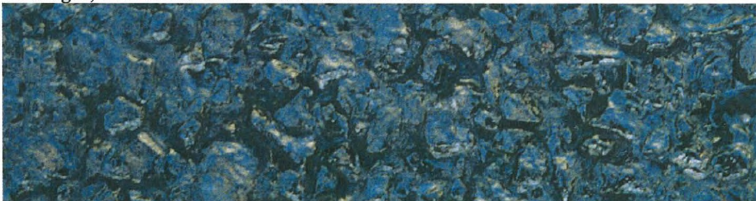
Coating C, total bitumen film thickness 13 microns
