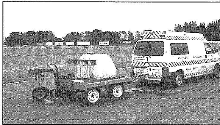
Figure 4.4 Norsemeter ROAR, an example of a variable slip skid tester.
