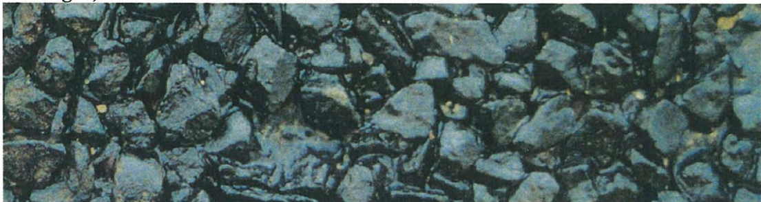
Coating D, total bitumen film thickness 110 microns
