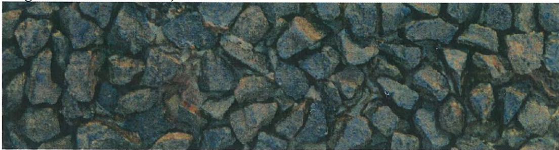
Coating A, total bitumen film thickness 1 micron
