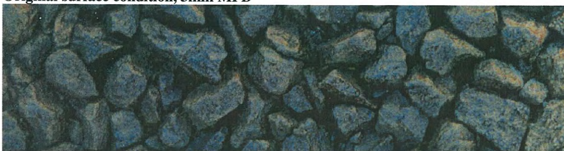
Coating A, total bitumen film thickness 1 micron
