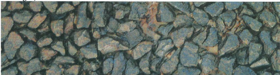
Coating B, total bitumen film thickness 4 microns
