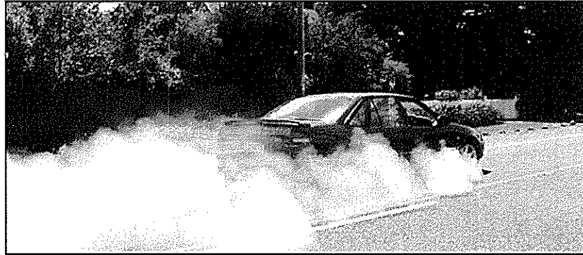
Figure 4.1 Instrumented test vehicle performing a dry surface emergency braking test.
