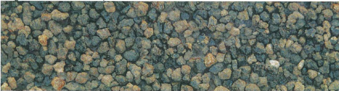
Coating A, total bitumen film thickness 1 micron
