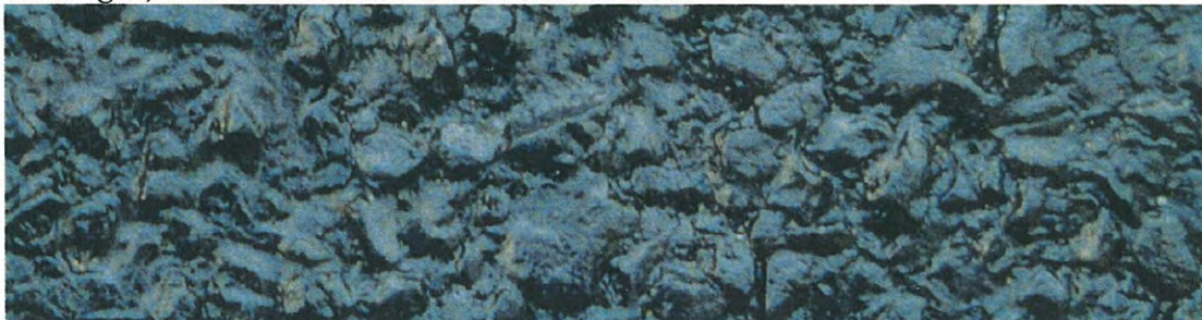
Coating D, total bitumen film thickness 110 microns
