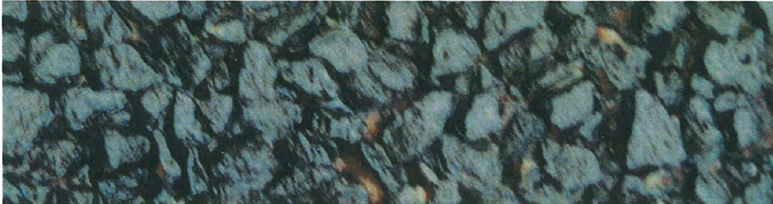
Coating D, total bitumen film thickness 110 microns
