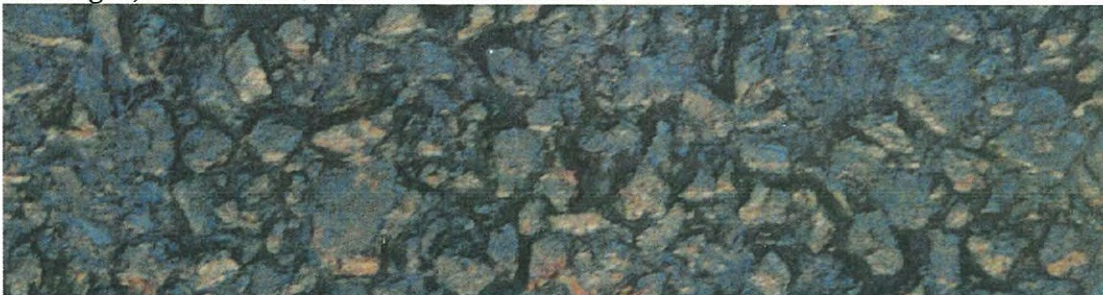
Coating B, total bitumen film thickness 4 microns
