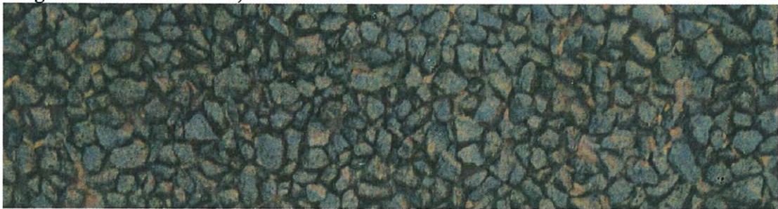
Coating A, total bitumen film thickness 1 micron
