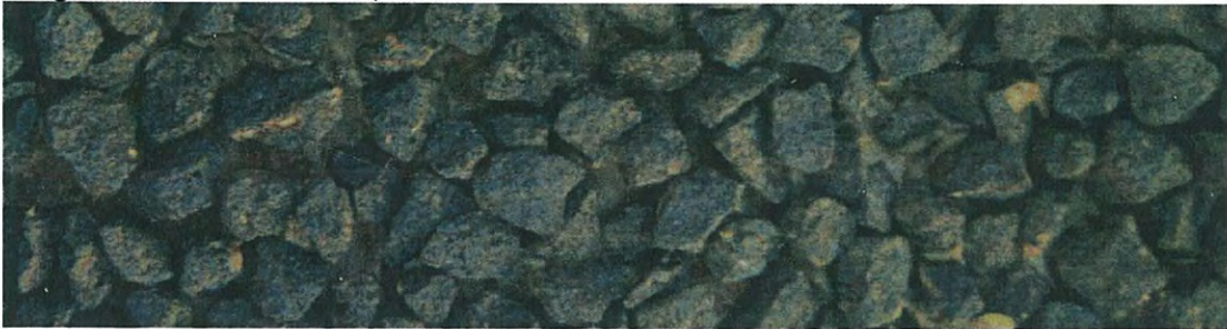
Coating A, total bitumen film thickness 1 micron
