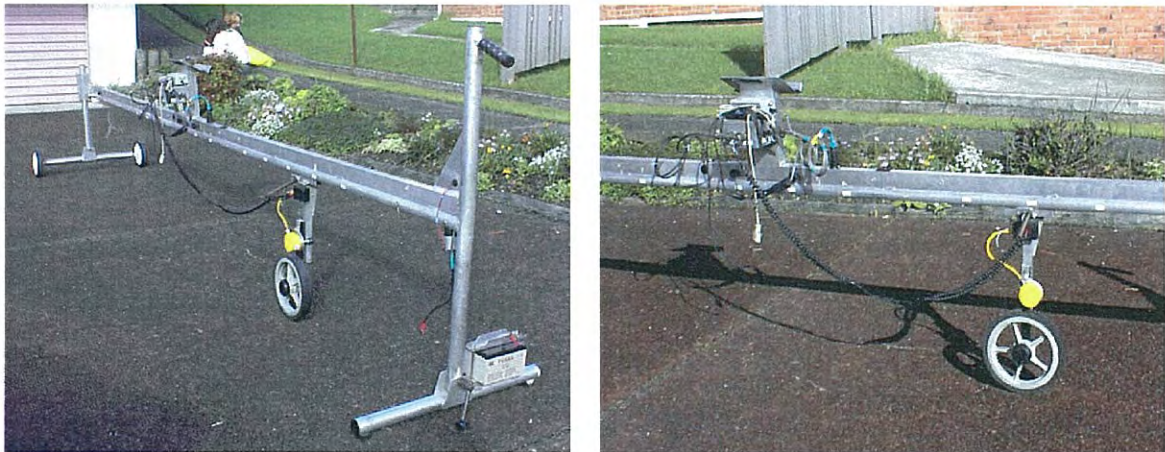
Figure 3.1: DCL Transverse Profile Beam
