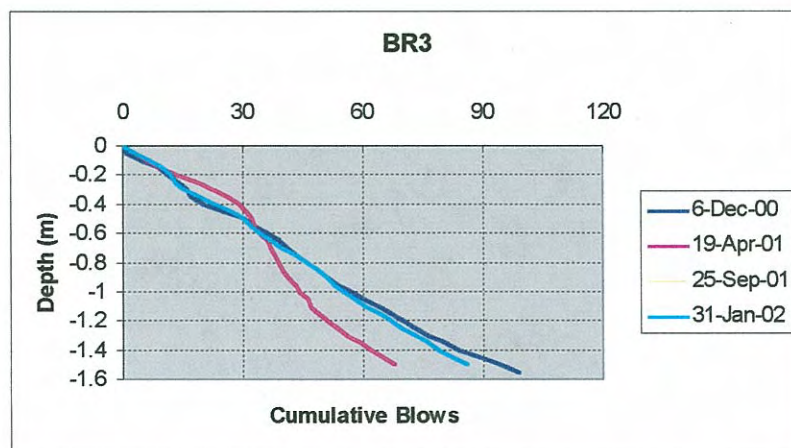
Figure 6.8(c) Subgrade DCP cumulative blows versus depth - Pit BR3.
