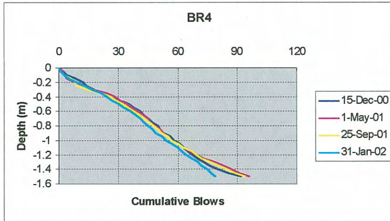
Figure 6.8(d) Subgrade DCP cumulative blows versus depth - Pit BR4.
