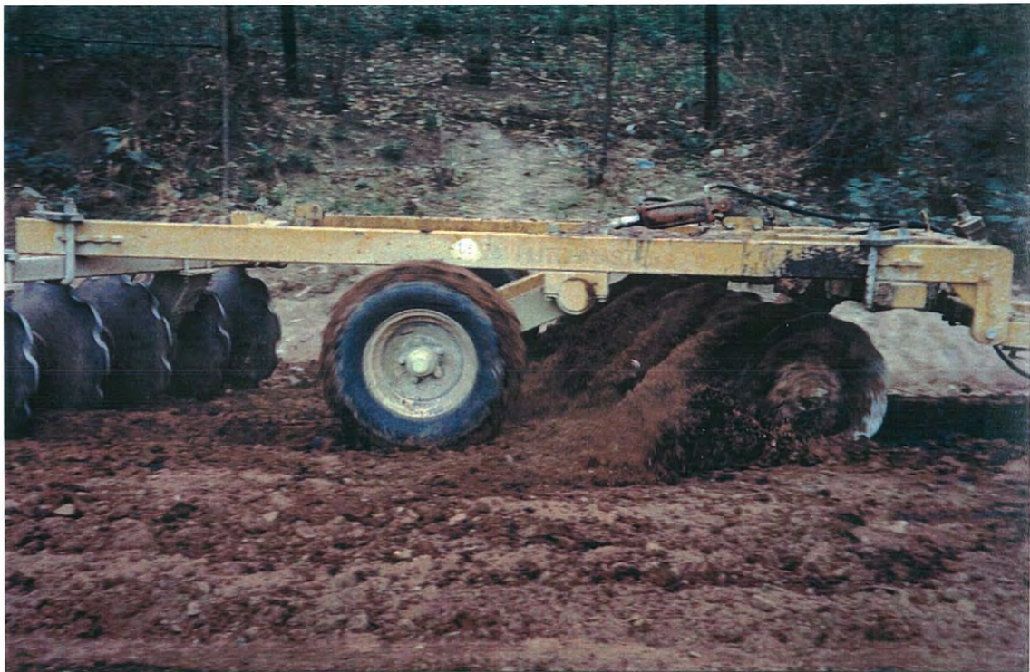
Figure 2-1 Agricultural disc mixing of emulsion D1621
