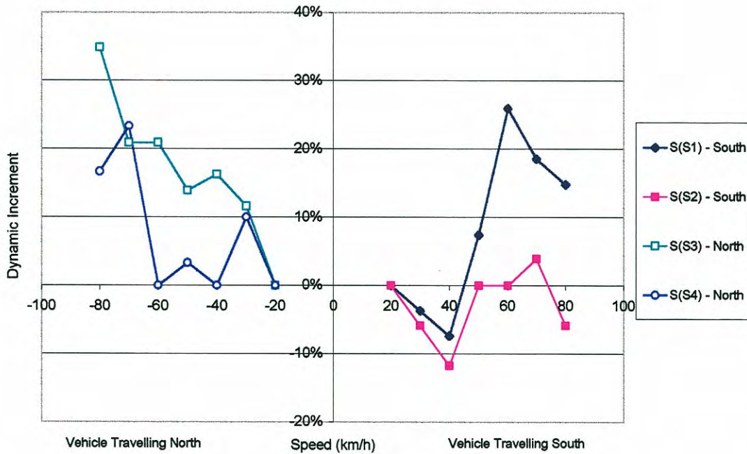
Figure 4.21 Dynamic increment plot for known vehicle travelling north to Tokoroa and south to Taupo.
