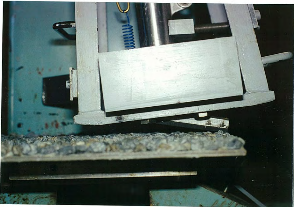
Figure 2.3 Chipseal surface stability test equipment.
