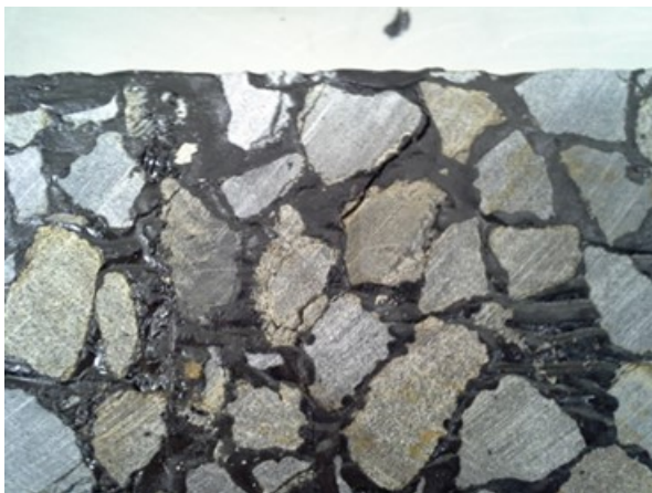
Figure 3.2 Photos illustrating cracks propagation as a result of repeated loading
