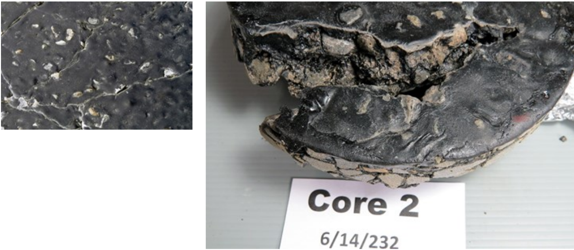
Figure 3.12 Cracked seal surface (left) and interior view of a crack showing the stripped seal (right)
