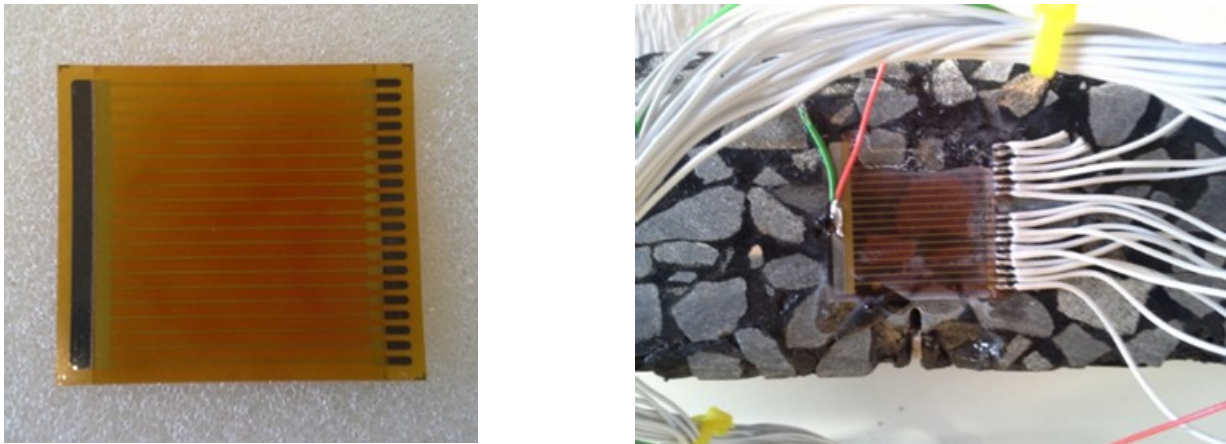
Figure 2.9 Crack propagation gauge (left); example of a gauge mounted on the side of a test beam (right)
