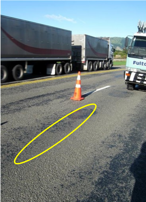
Figure 2.10 SH1 Otaki site showing position of slab 1 taken for preparation of fatigue test specimens
