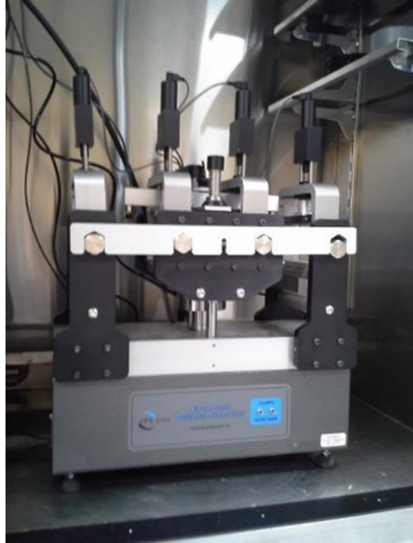
Figure 2.13 IPC Global's four- point bending apparatus with beam mounted (left). The load is applied downwards from the neutral position so the bottom surface is in tension
