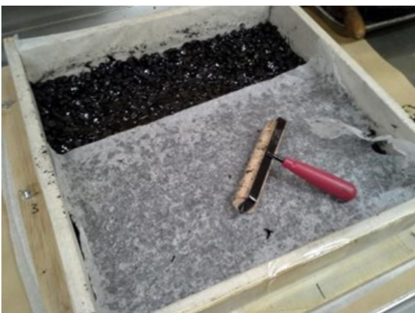
Figure 2.5 Roller compaction of the first layer (left); construction of the subsequent layer (right)
