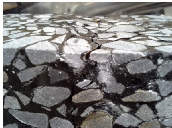
Figure 3.2 Photos illustrating cracks propagation as a result of repeated loading
