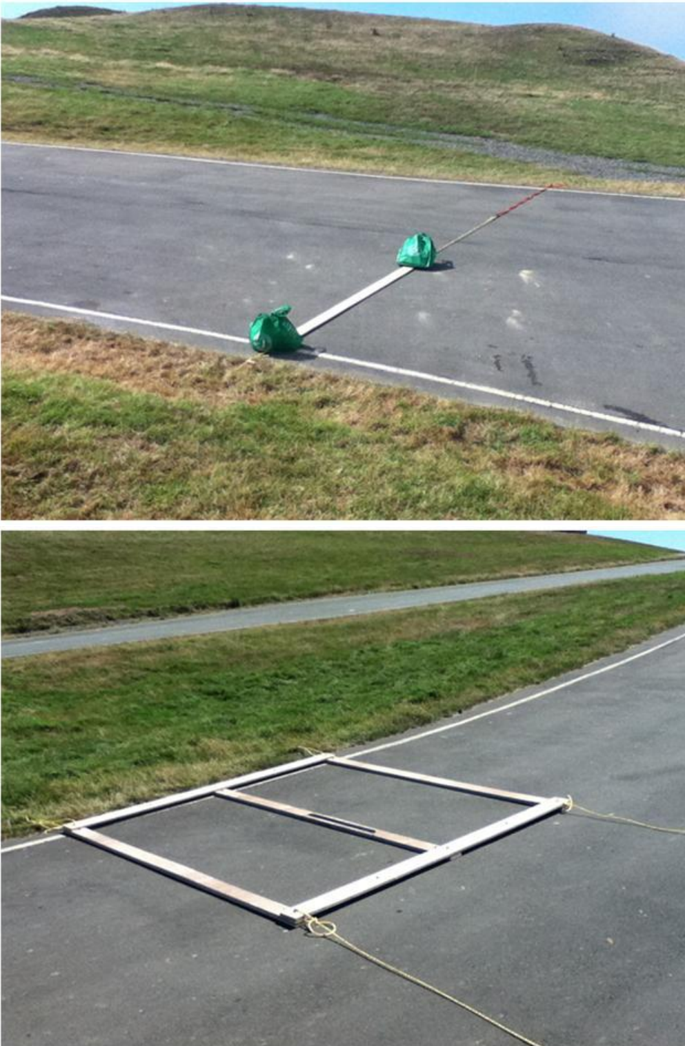
Figure 5 Views of single and multiple roughness elements
