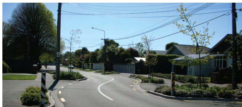
Photo 6.3 – Traffic calming by road narrowing, Christchurch (Photo: Megan Fowler)
