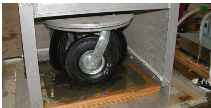
Figure 1 The Auckland accelerated polishing device developed as part of the research
