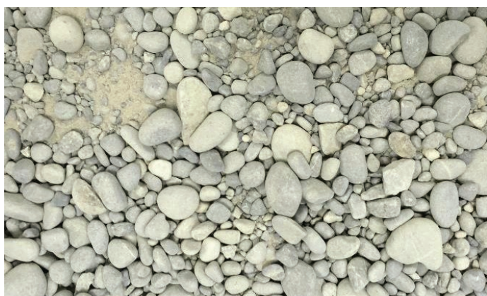
Aggregate sample before placement in triaxial cell Dry sample, 1.99tm-3
