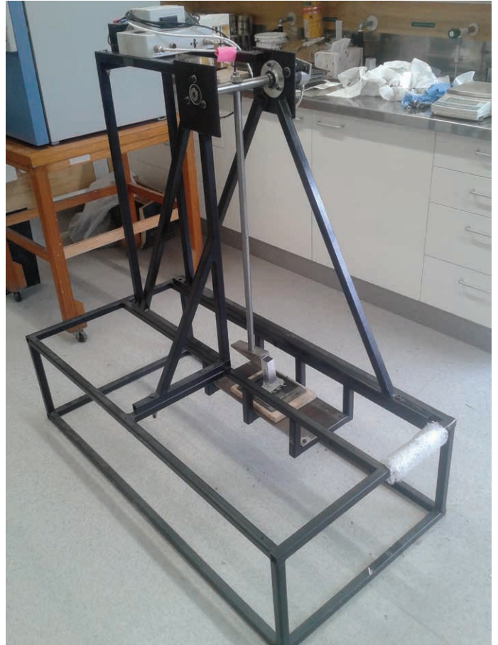
Opus Research pendulum tester with chipseal sample in place
