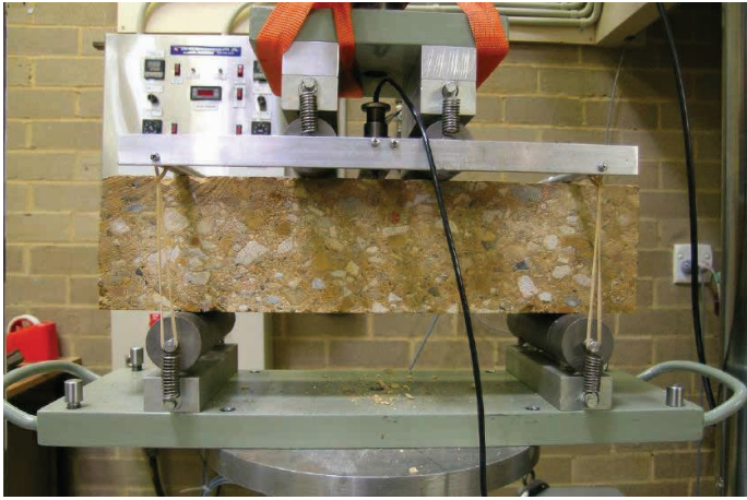
Flexural beam test Source: Austroads (2008)
