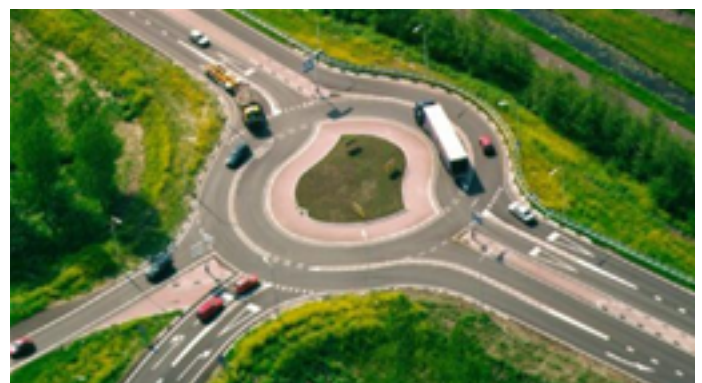
A turbo-roundabout in The Netherlands, showing the typical layout
