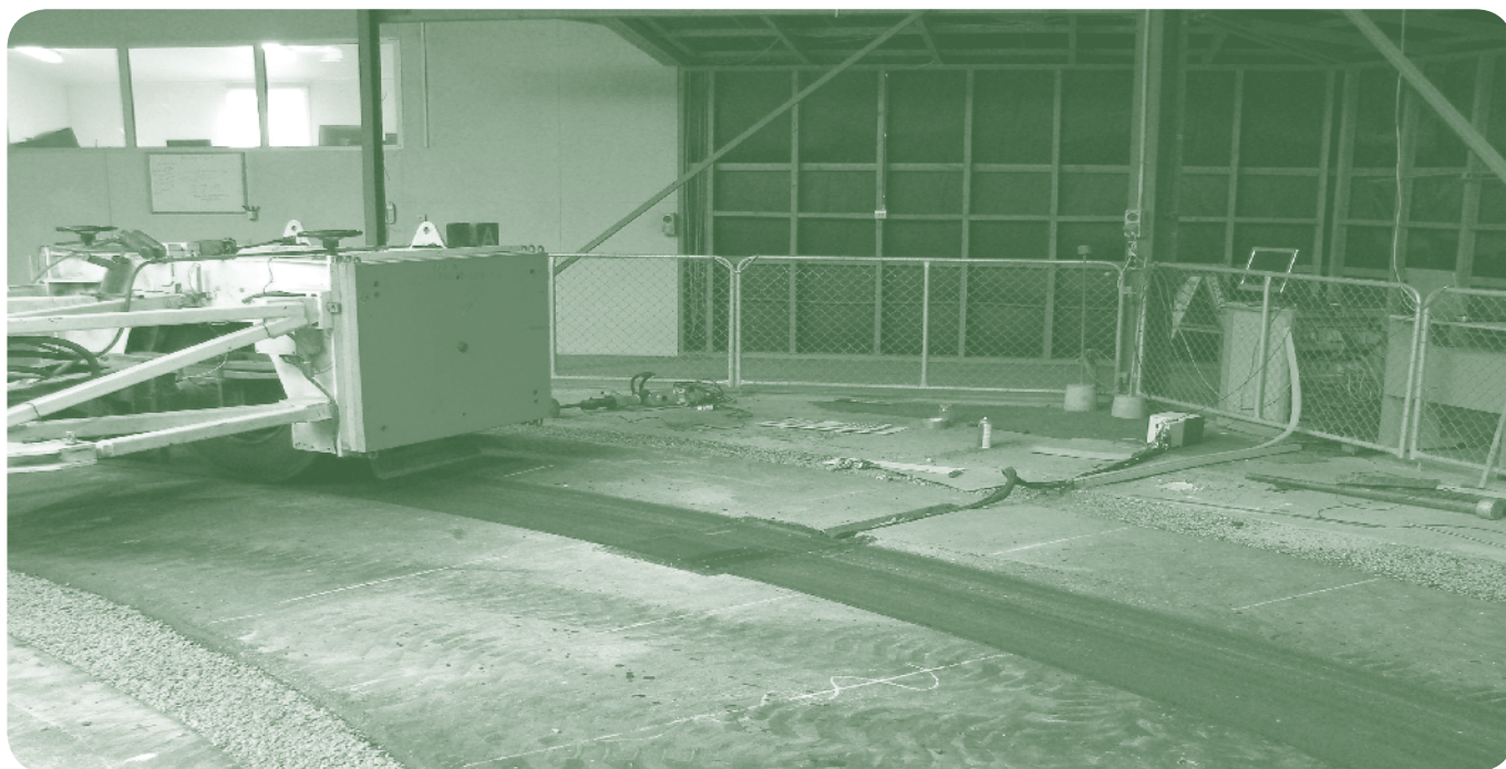
The apparatus designed to accurately measure tyre-road contact stress distributions.
