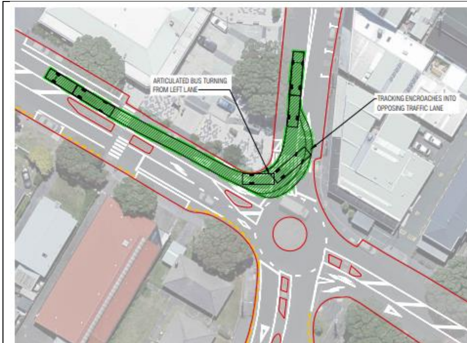
Figure 3: Existing geometry at an intersection. The left-hand turn lane is unsuitable for articulated buses. Also, buses turning left from the straight/right lane would put undertaking cars or bicycles turning left at risk.
