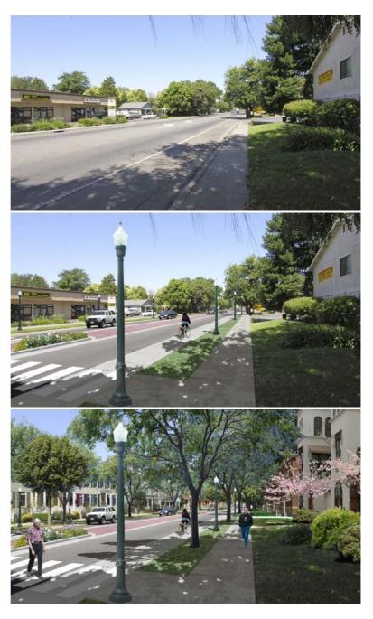
Step 1. Addition of street lighting, medium strip, low level planting, cycle lane, widened footpath, pedestrian crossing.
