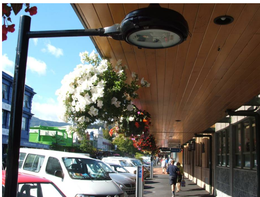
Photo 5. Purpose-built under-veranda footpath street lights for Nelson CBD. Also removal of individual parking meters and control of shop sandwich board sign clutter.
