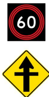
Figure 3. Example of an AWRS (with pulsing roundel) and supplementary warning sign (PW-9 intersection layout static panel) (Source: 'ISZ signs' section of ITS design standard: Active warning and regulatory signs).
