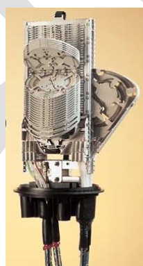
Figure 9. Tray mounting system layout.
