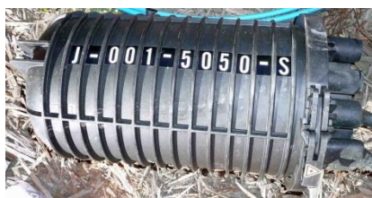
Figure 7. Dome labelling example: J-001-5050-S.
