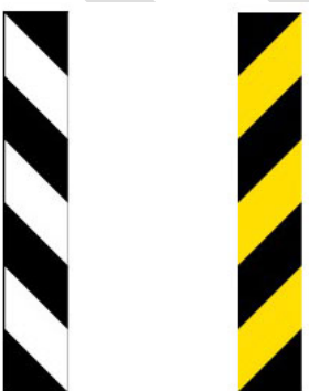
Figure 10. W20-5.1 and W20-5.2 bridge end markers
