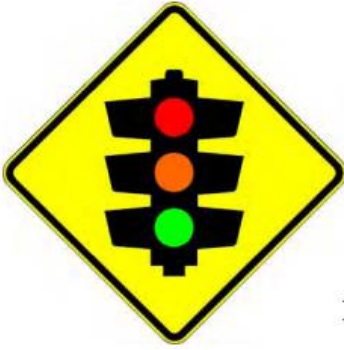
Figure 8. W10-4 sign traffic signals ahead
