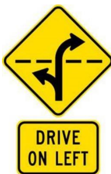
Figure 3. W14-11.1 drive on left sign with supplementary sign
