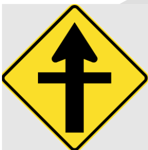
Figure 2. WJ2A Intersection layout static panel
