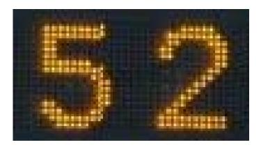
Hybrid A typical hybrid EWS utilizes both flip disk and either fibre optic or LED technology. Each flip disk has a hole for light to pass through. The light is generated by a fibre optic bundle or LED pixel. When the pixel is activated the disk is flipped, allowing light to pass through the hole while displaying the reflective side of the disk to traffic. When the pixel is off its reflective surface is rotated, or flipped, blocking the light source.
