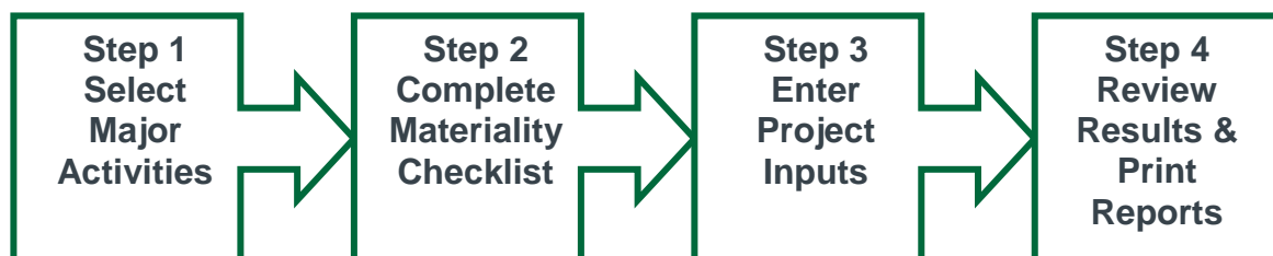
Figure 8.1-The four steps required to estimate the GHG emissions for a road project.
