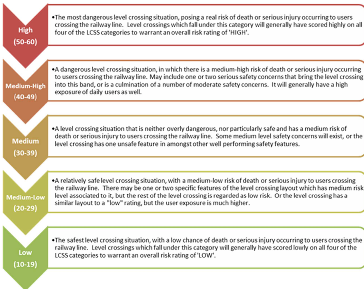
Figure 7: Level crossing safety score risk bands
