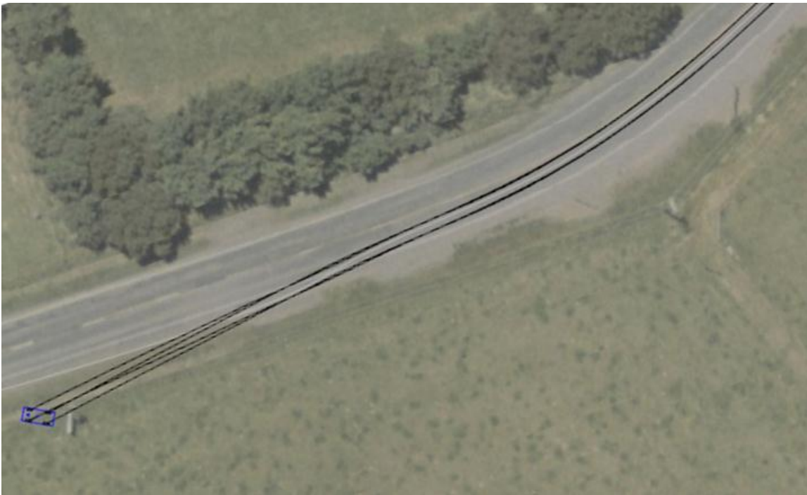
Figure 18: Simulated Vehicle Path – PC-Crash
