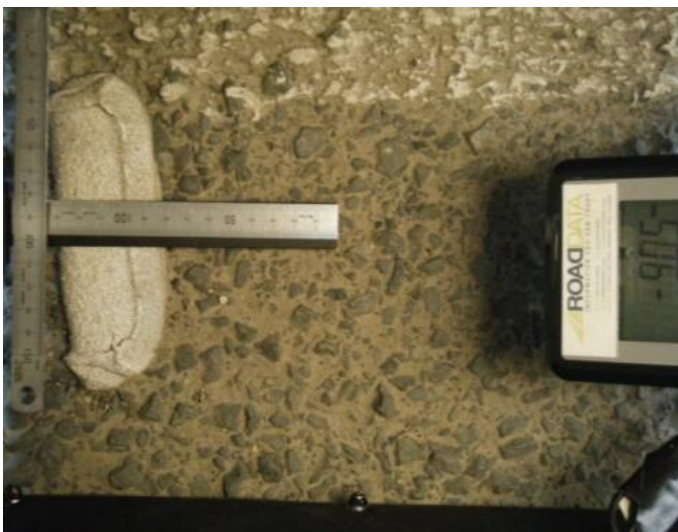
Figure 8-2: ATPM ribs, with good rib height, in need of cleaning (Mackie, 2009a, page 15)
