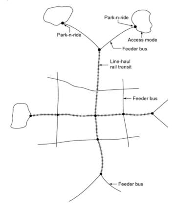
Figure 3.3 Relationship of feeder services to the rest of the network (source: Victor and Ponnuswamy 2012)
