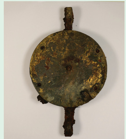
A British made guilt Salter's scale spring balance, Silvester's patent, which would've been capable of weighing up to 200lbs (approximately 90kg).
