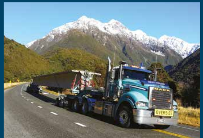
The Super-T beams were transported to site one at a time via Arthur's Pass
