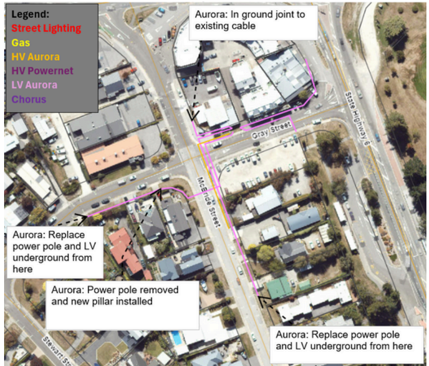
Stage 1 of the Gray-McBride works involves undergrounding our power network. Note: Service locations are indicative only.
