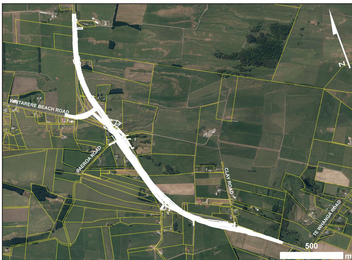
Figure 2: Detail of the proposed highway realignment showing divergence from current SH1 alignment, connections to existing roads and affected land parcels. Poroutawhao School turning lane not shown.
