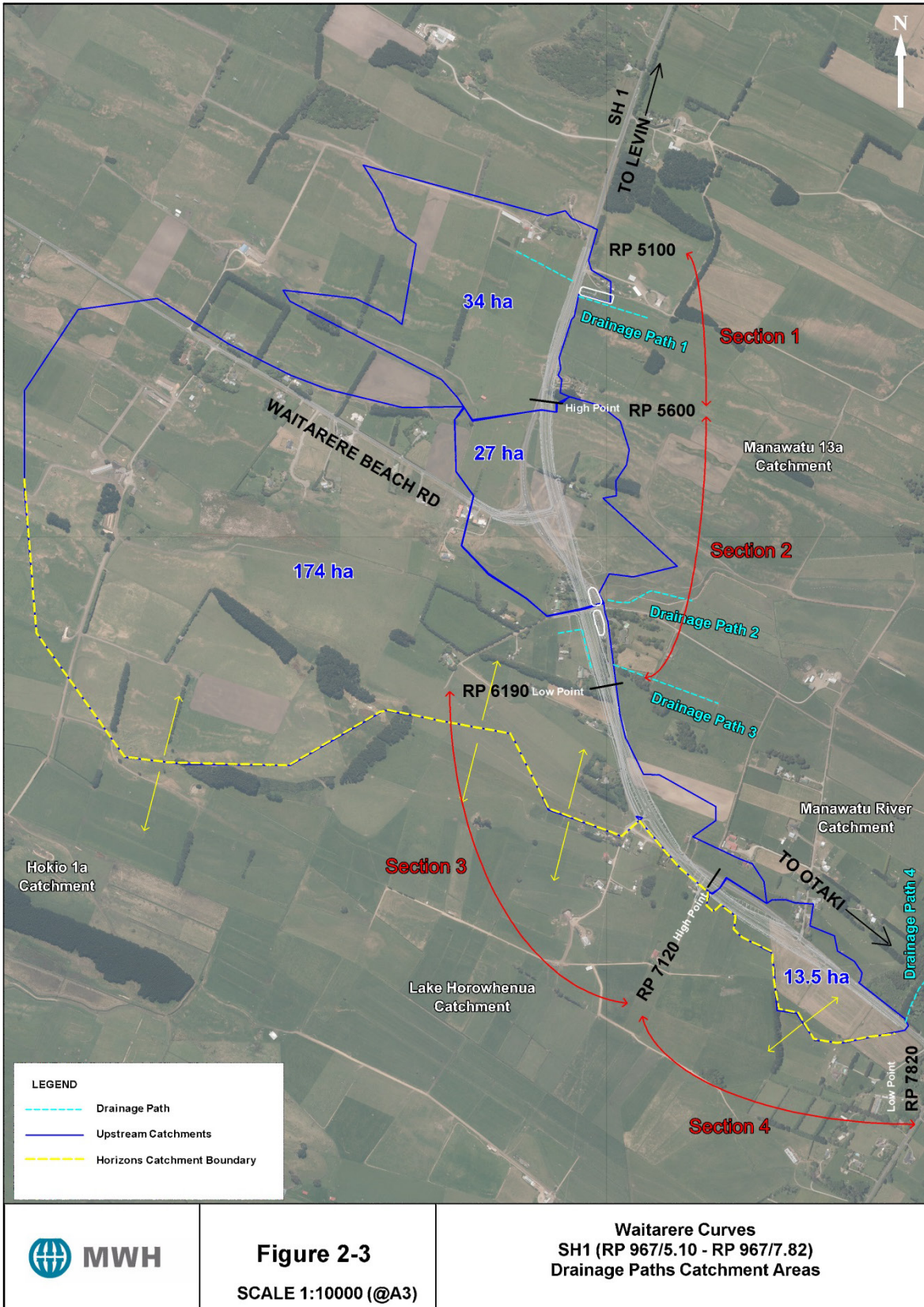
Figure 2-3: Drainage paths and catchment areas
