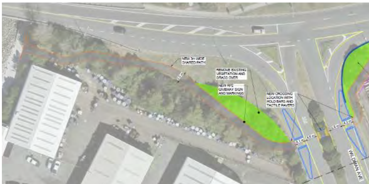
Figure 3: New Connection from the Existing SH6 Underpass and Maitai River Shared Path to Wildman Avenue
