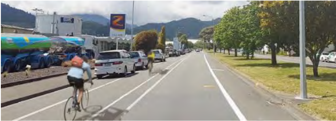
Figure 1: Option 1 Do Minimum Photo Simulation with 0.5m Buffer Between Cyclist and Vehicle Lane
