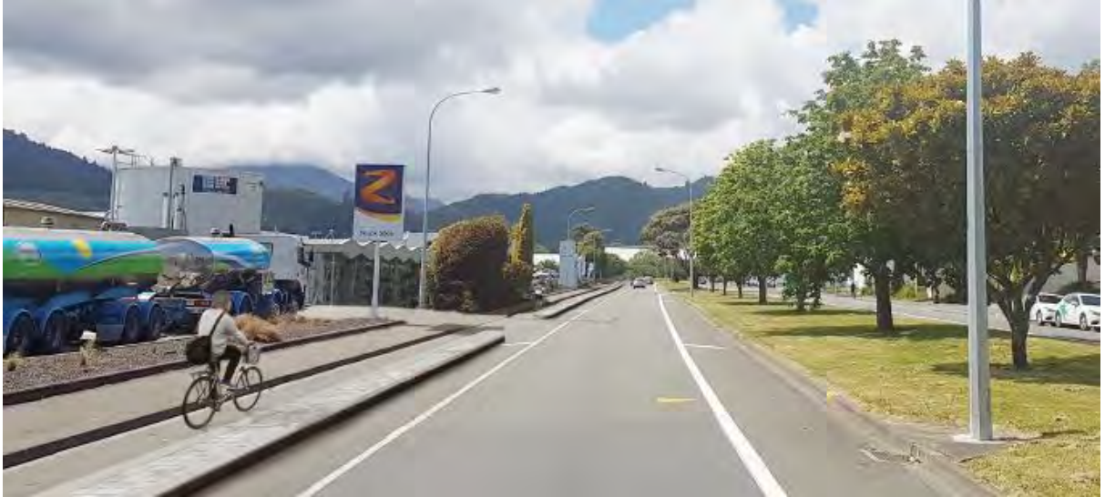
Figure 4: Option 2 Separated Cycle Lane photo simulation with solid separator island between cyclist and vehicle lane
