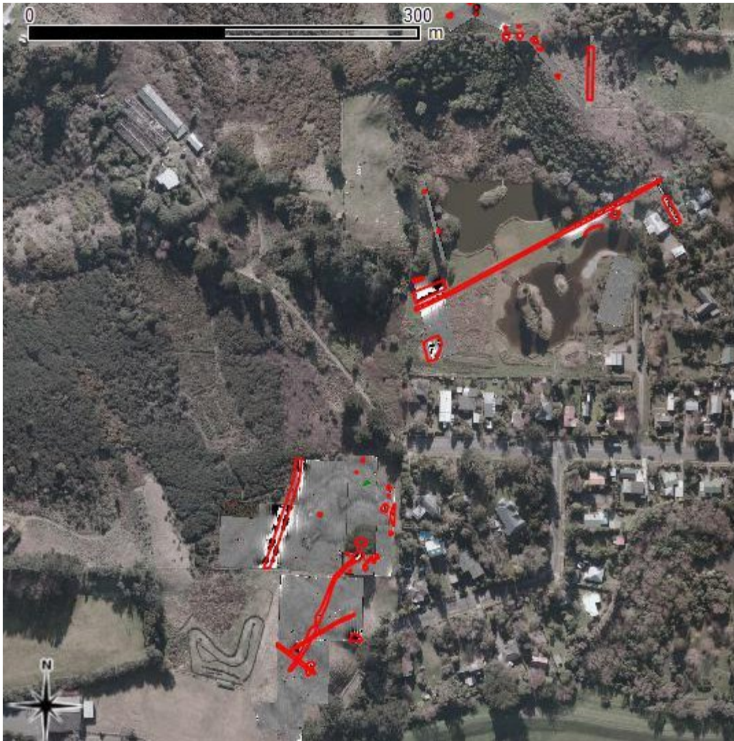
Figure 1: All geomagnetic survey areas and magnetic anomalies (red).
