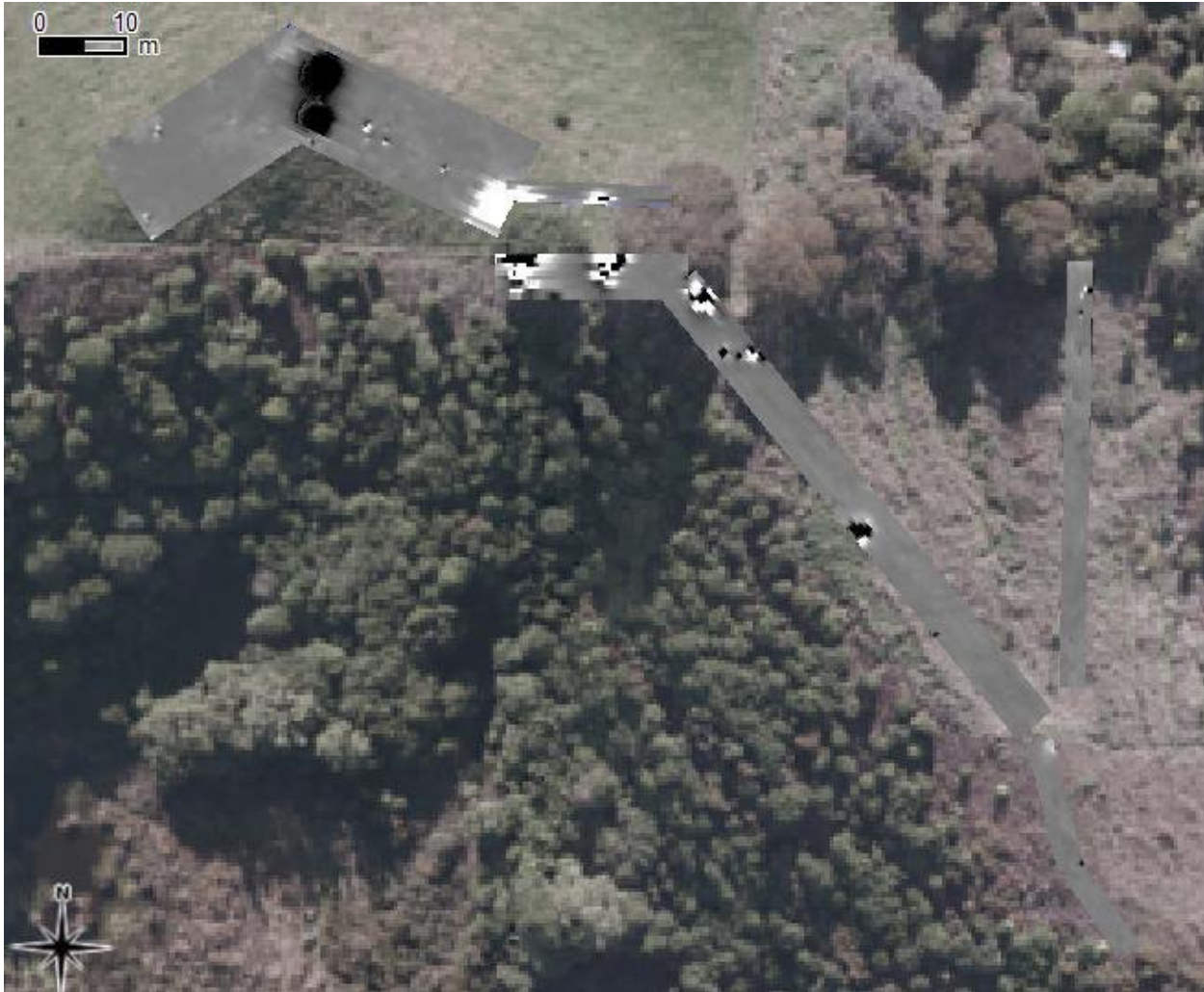
Figure 2: Geomagnetic survey areas in grey overlaid onto aerial photograph.
