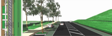
Parking kerbside and trees behind footpath
