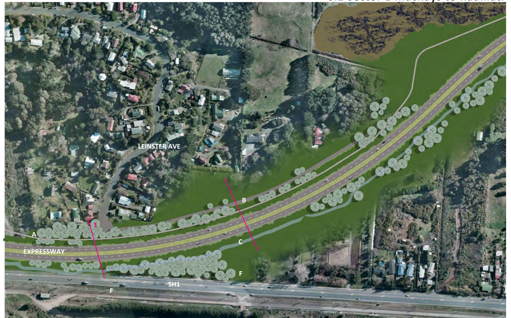
Figure 128 At the Leinster Ave area showing landscape integration proposals and below sections describe the landform manipulation to provide visual and noise separation
