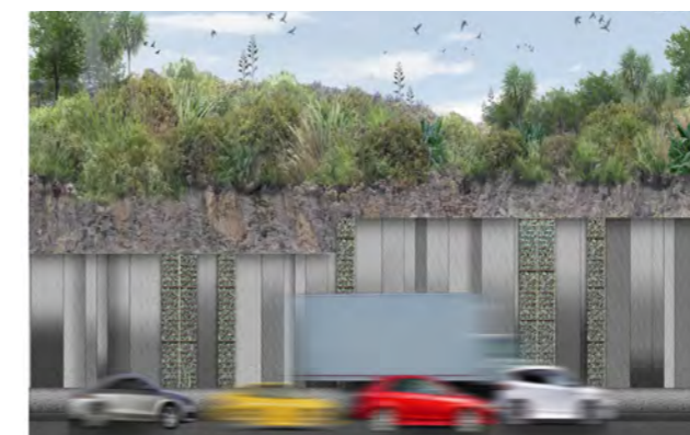
TYPE B: Gabion basket type wall - maybe gabion facing with solid wall. TYPE C: use of standard slipform concrete barrier. For both types the land form behind the wall will be built up to mask the wall height from the adjacent properties and this slope planted.
