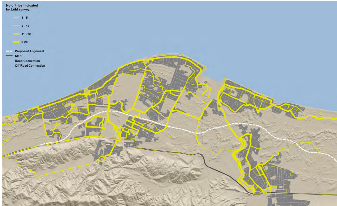
Figure 44 above shows mapped cycling results from the Local Area Movement Survey (LAMS) which describes the relative frequency with which people cycled along either streets or other paths. The figures are derived from the survey and show the number of respondents that used the route in a week. Notable (like the walking results) is the heavy use of Waikanae River paths, Wharemauku Stream path as well as the movement between Waikanae and Paraparaumu utilising the Waikanae River walking bridge. Also of note are movements across the Expressway route (dashed white line).
