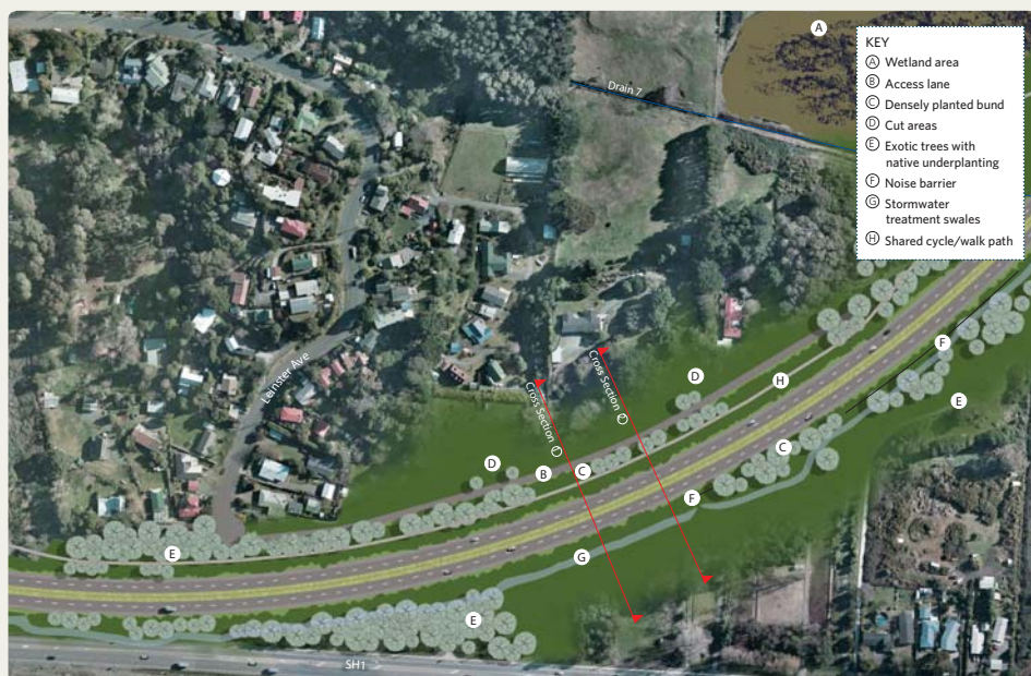
The indicative mitigation design includes the integration of landforms - bunds - to buffer residential properties from the expressway. A combination of dense native underplanting and taller exotic trees matches the existing planted landscape. Noise barriers will also be incorporated in some areas with their design to reflect the nearby property's purpose. The wetland areas will be retained and will have a stormwater management function.
