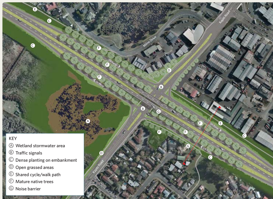
The indicative mitigation design for the area around the interchange will consider the architecture of the bridge, the landscape design of the ground around the structure, and the way in which people move around and experience the bridge from below. This interchange is also a key 'gateway' point for expressway users and the way this is experienced by these users will be considered.
