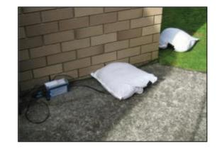
Setup comment: Dwelling transducer placed on exposed aggregate patio attached to house and sandbagged.
