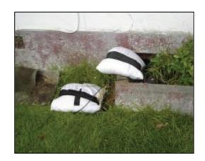
Setup comment: Dwelling transducer placed on concrete parapet of sub-floor access point and sandbagged. Ground transducer placed in lawn immediately adjacent, with ground spikes, and sandbagged.
