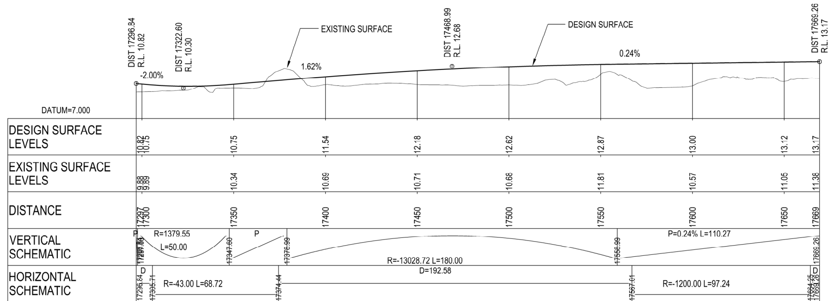
LONGITUDINAL SECTION - NORTH BOUND ON-RAMP
