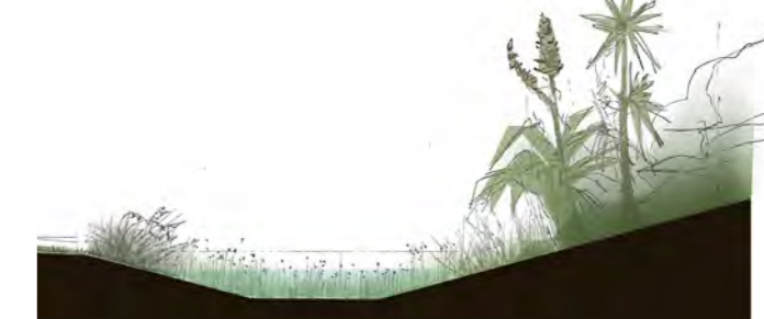
Figure 107 Storm water swales
