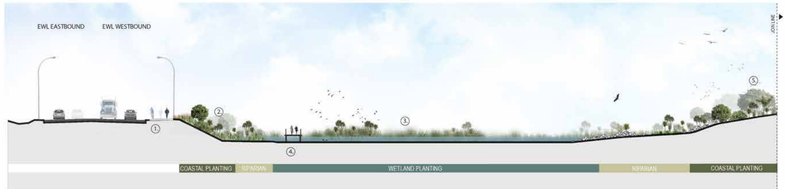
COASTAL EMBANKMENT - 2D SECTION (A6) 3450 SCALE 1:500
