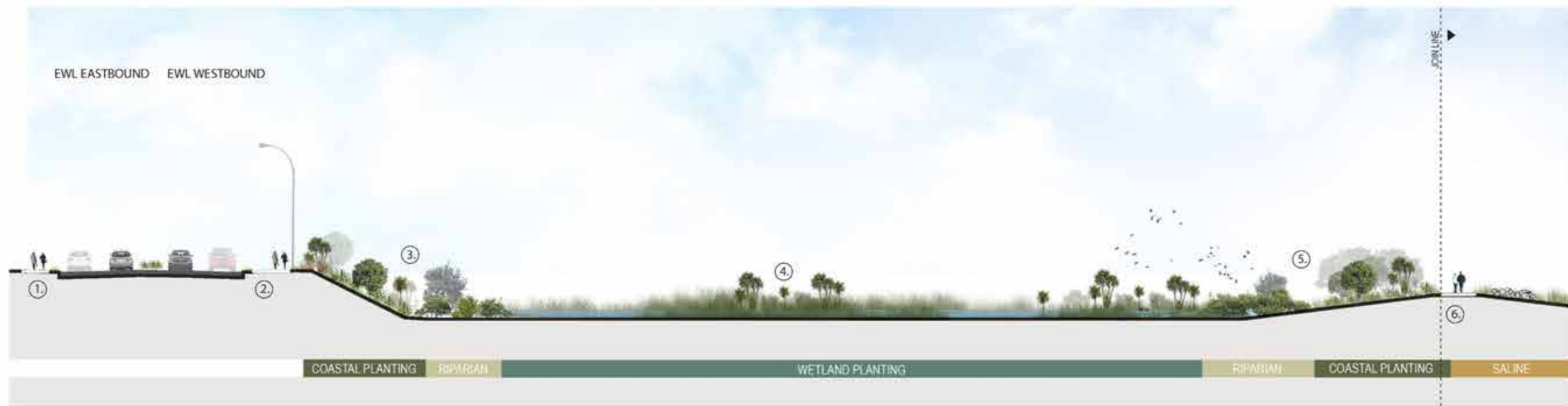
COASTAL EMBANKMENT - 2D SECTION (A5) 2950 SCALE 1:500
