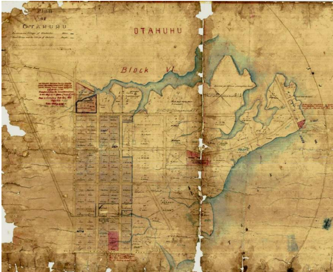
Figure 6-3: SO 678 showing the grid of streets and one-acre town allotments laid out for the Fencible settlement at Ōtāhuhu with small farms to the east.
