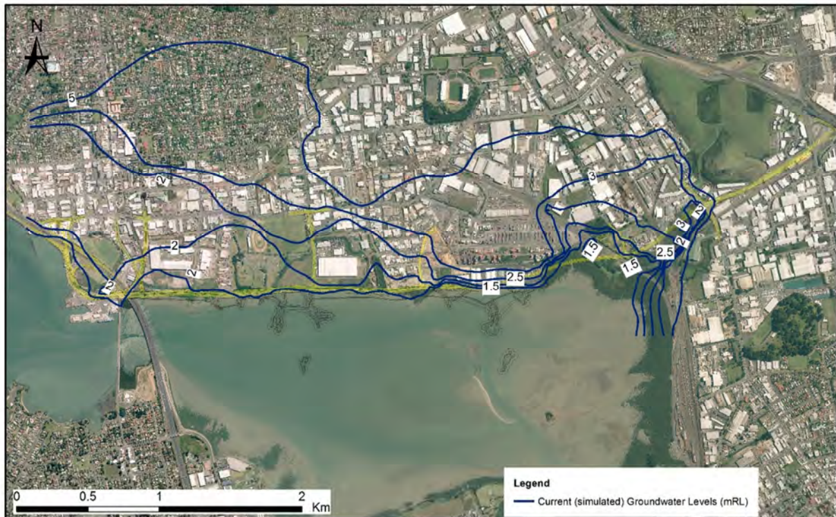
Figure 4-8: Simulated water table elevations (contours in metres RL)
