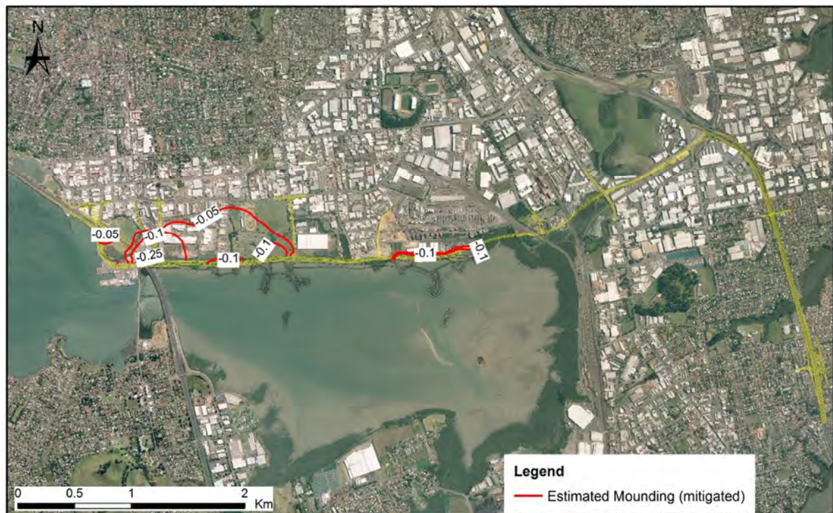
Figure 5-8: Change in groundwater levels as a result of the Project (mitigated) (contours in metres; negative number indicates groundwater level rise)
