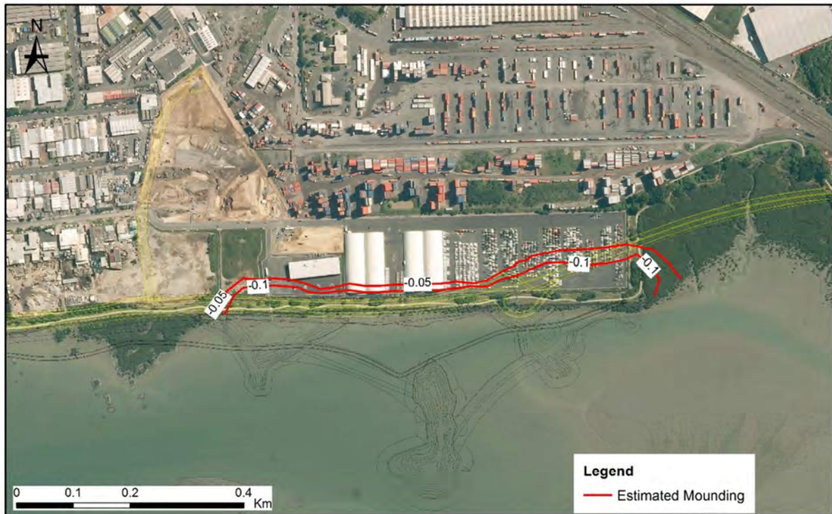
Figure 7.4: Sector 2 East: Change in groundwater levels as a result of the Project (contours in metres; negative number indicates groundwater level rise)
