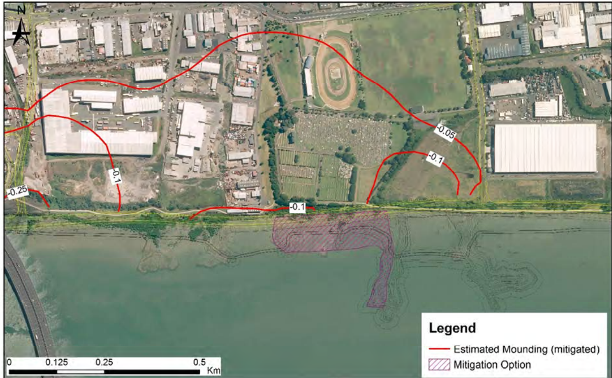
Figure 7.6: Change in groundwater levels as a result of the Project (mitigated) (contours in metres; negative number indicates groundwater level rise)
