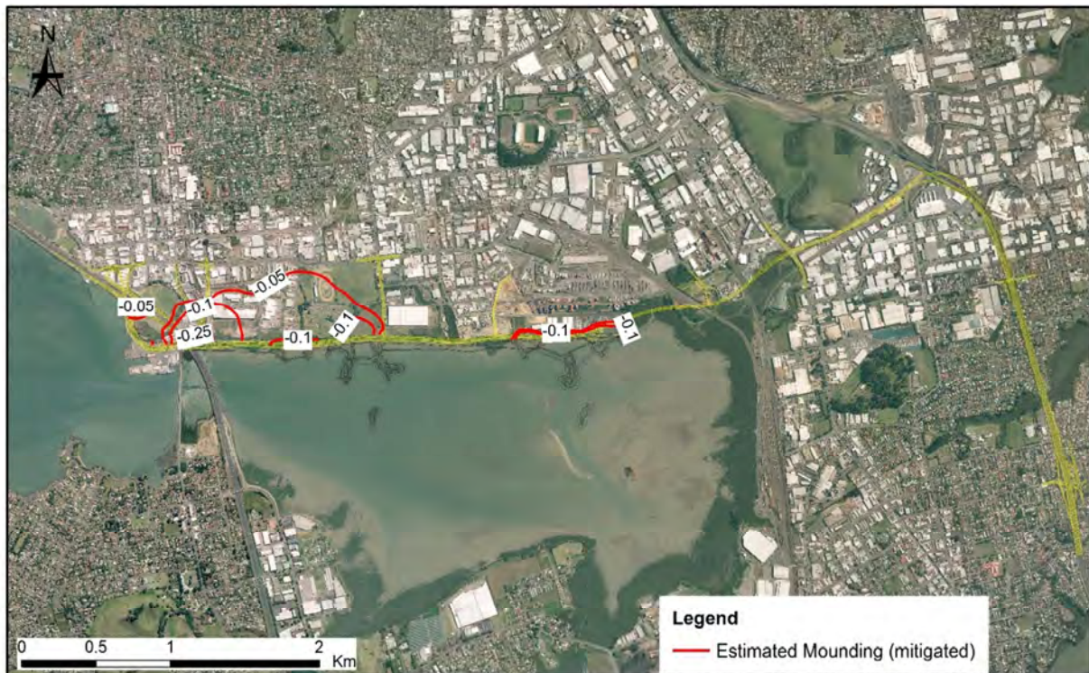
Figure 7.6: Change in groundwater levels as a result of the Project (mitigated) (contours in metres; negative number indicates groundwater level rise)
