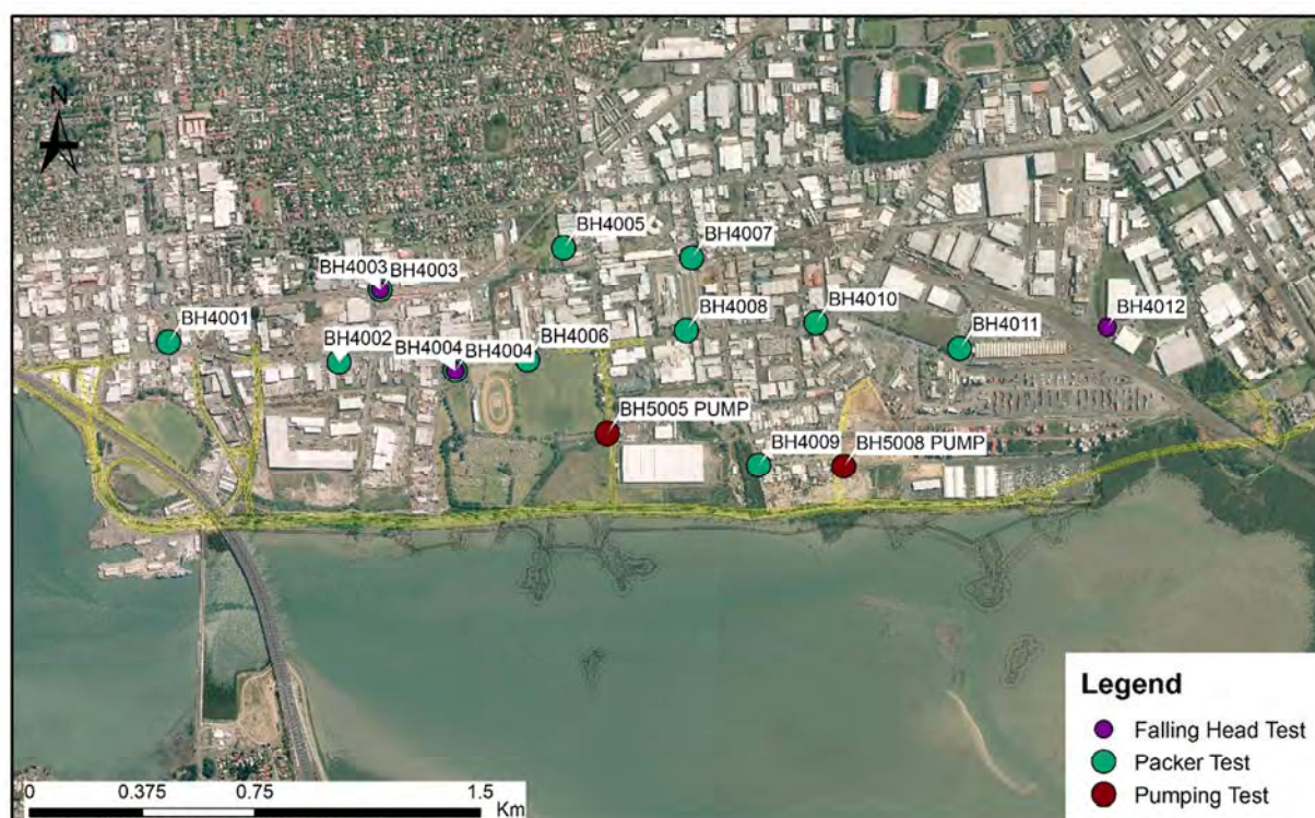
Figure 4.2: Permeability testing locations
