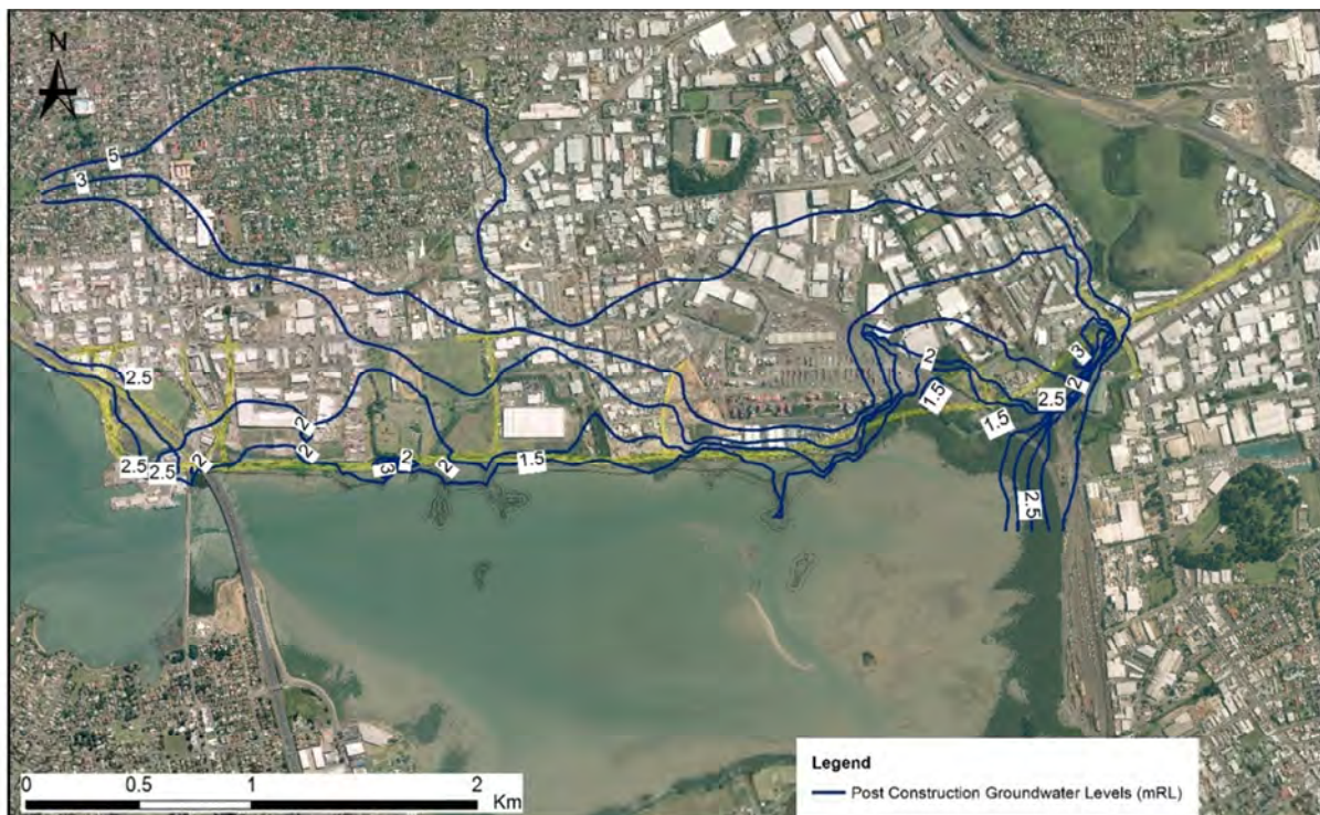
Figure 5-4: Modelled groundwater levels after Project construction
