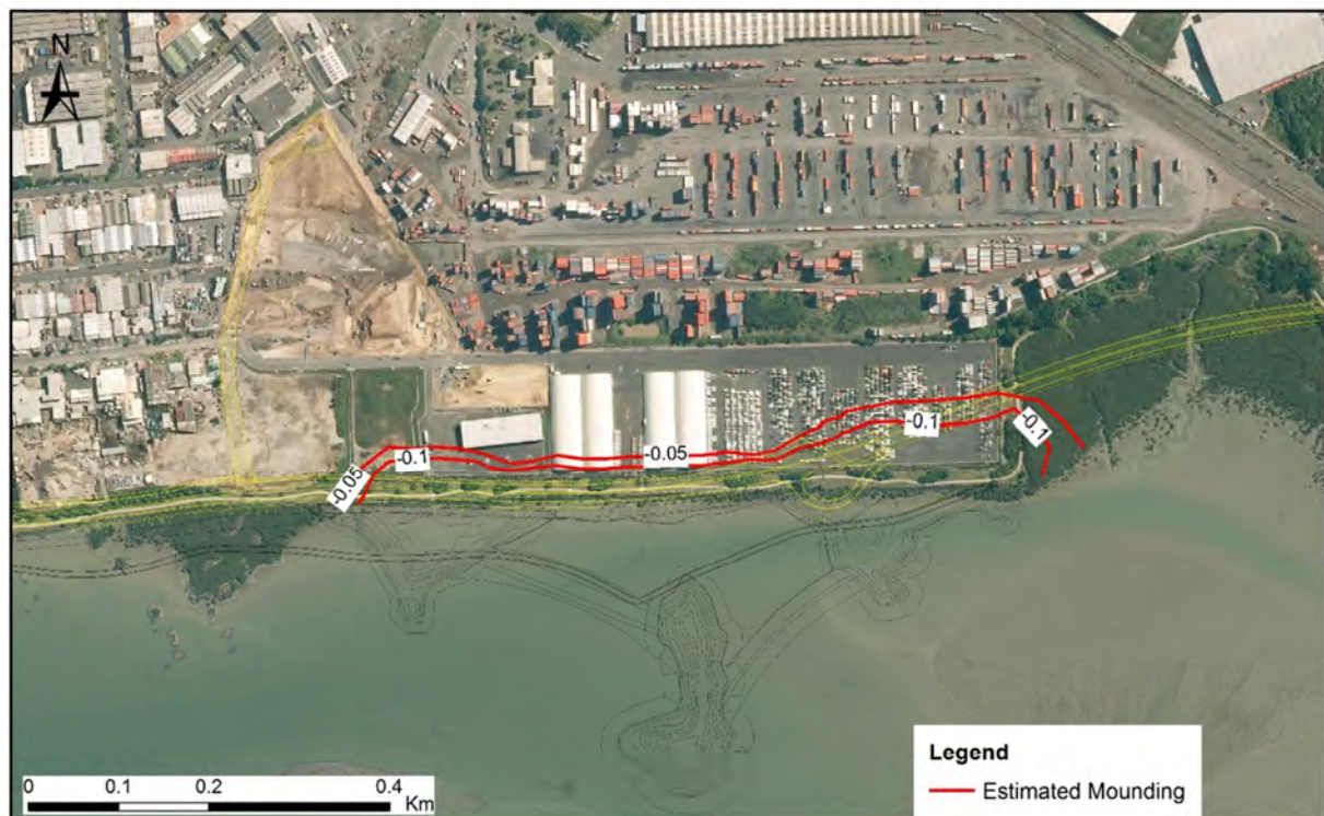
Figure 5-9: Sector 2 East: Change in groundwater levels as a result of the Project (contours in metres; negative number indicates groundwater level rise)
