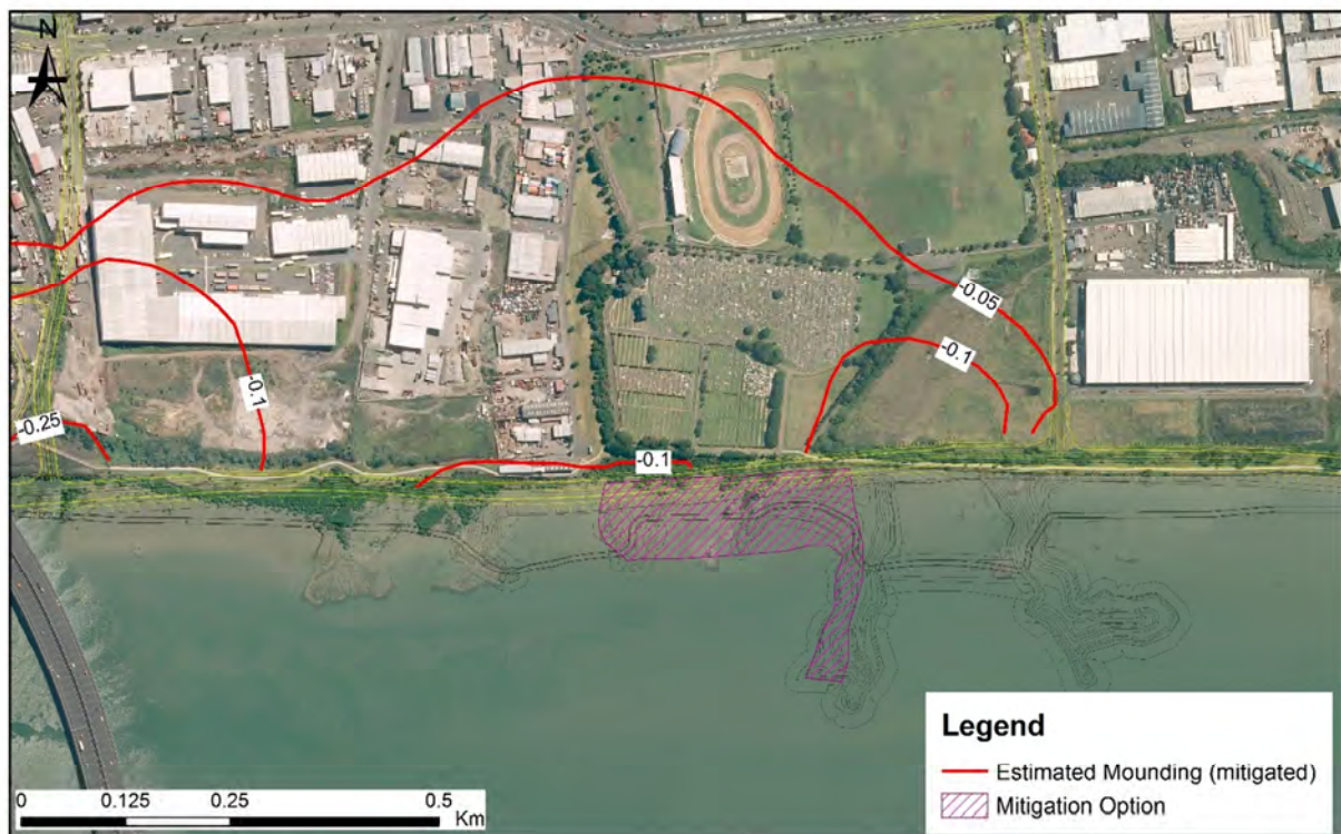
Figure 6-1: Sector 2 East: Mitigated change in groundwater levels as a result of the Project (contours in metres; negative number indicates groundwater level rise)
