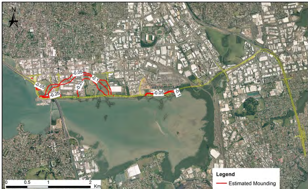
Figure 5-5: Change in groundwater levels as a result of the Project (unmitigated) (contours in metres)
