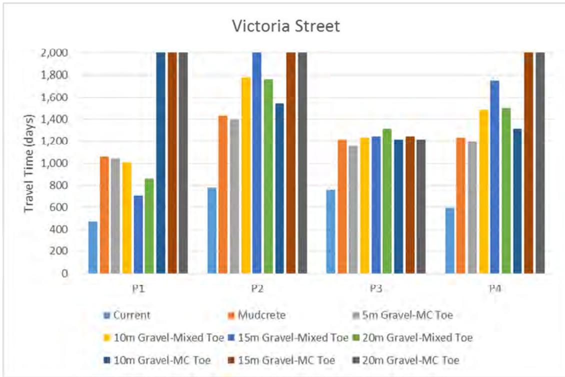
Figure 5.3: Victoria Street section: travel times results for gravel core
