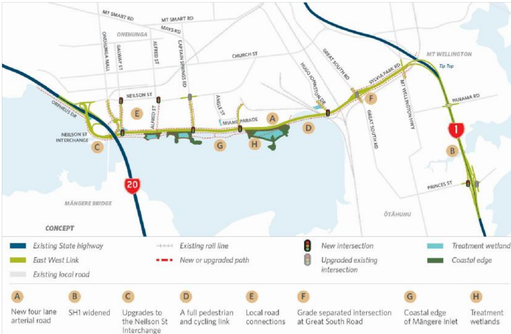
Figure 1: Key components of the project
