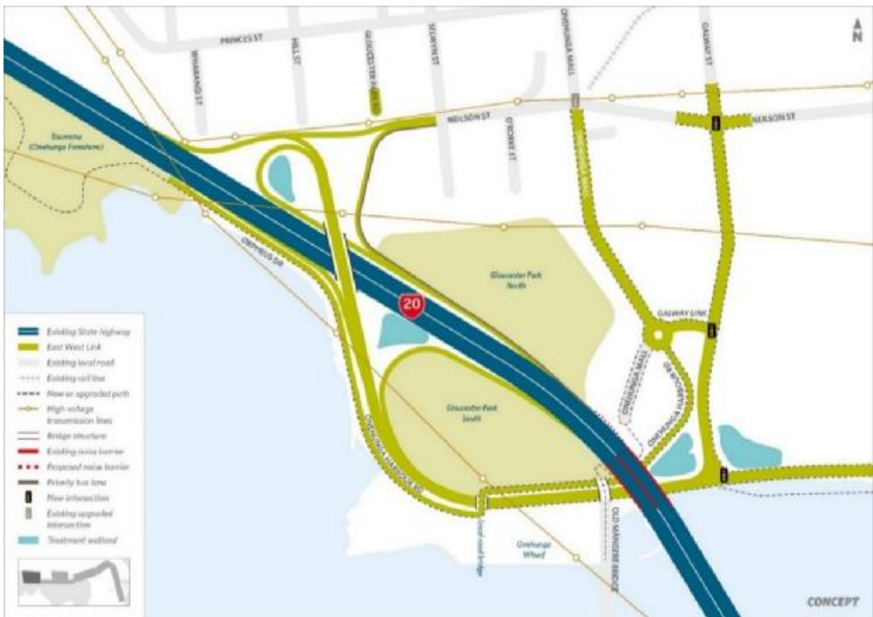
Figure 2: Neilson Street interchange indicative layout
