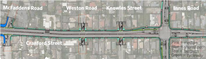
The design of Cranford Street between the Christchurch Northern Corridor connection and Innes Road is being upgraded to include four traffic lanes and a central median.
