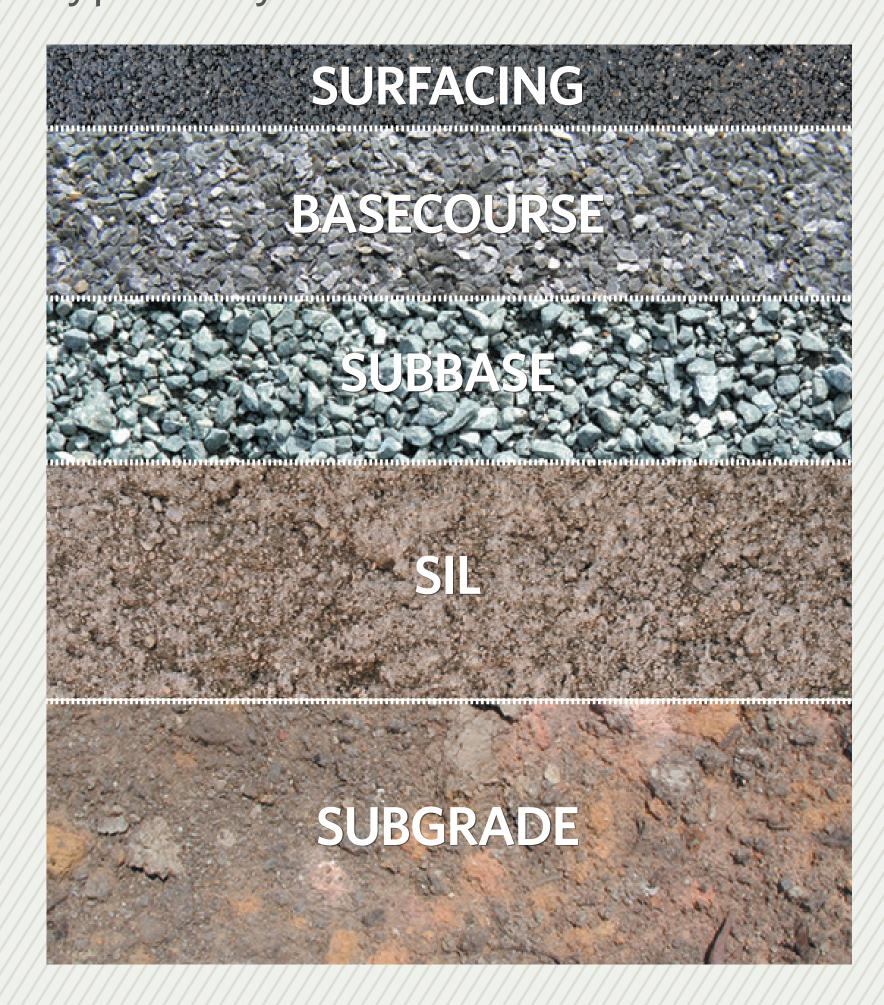
**Surfacing:** This varies depending on the road usage and traffic volumes, but the types of surfacing we have on this project include chip seal, asphaltic concrete and the smooth surface of open graded porous asphalt (OGPA).
