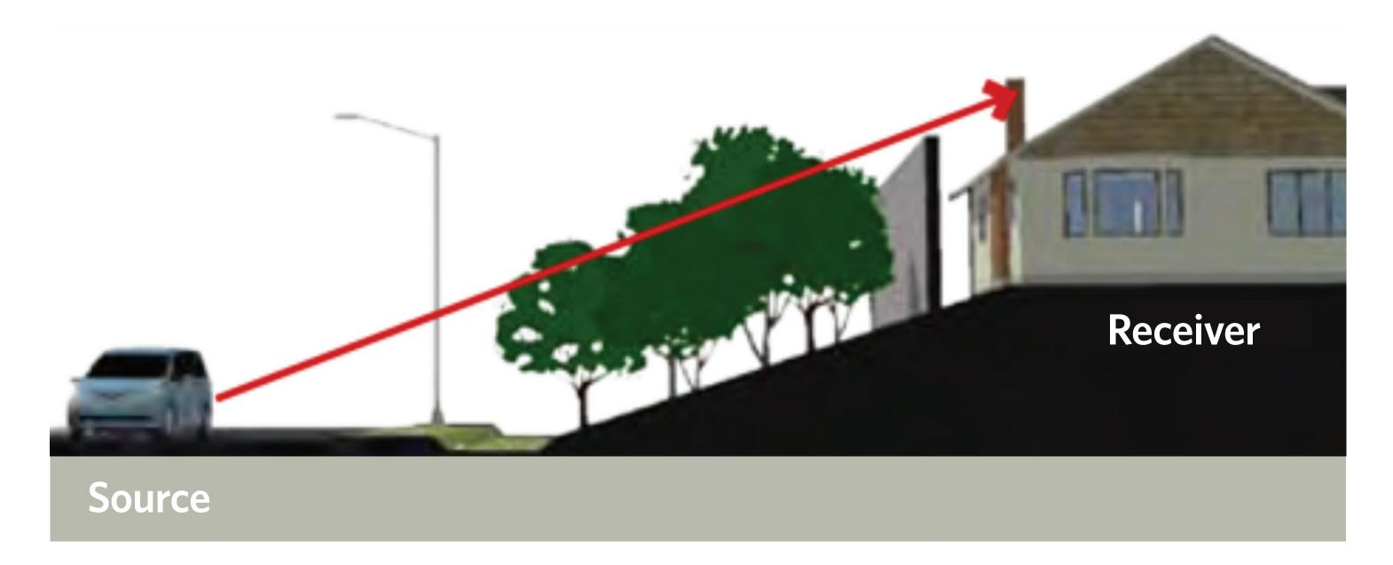
The height of a noise barrier is a key parameter. Generally the higher the barrier, the greater the level of noise reduction. As a general rule, a noise barrier should at least be high enough to block the line-ofsight from a house to the engines of vehicles on a road.
